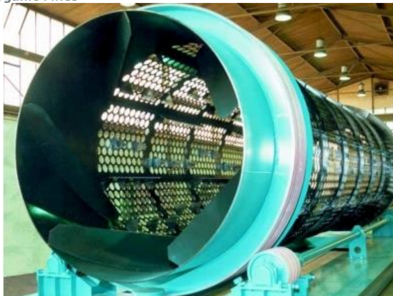
Figure A2-1: Trommel Screen Used to Separate Lighter, Combustible Material (i.e. 'Overs') from 'Organic Fines'
